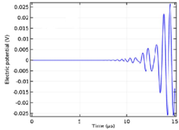
**Figure 14.** Received signal for 50 degrees beam angle
