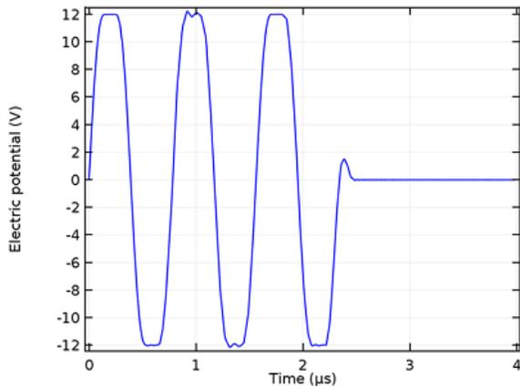
**Figure 9.** Excitation signal for investigating effect of pipe diameter
