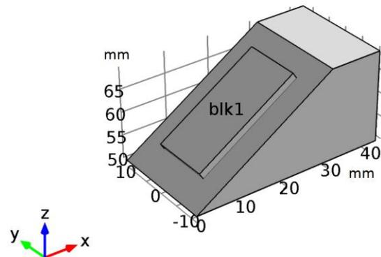
**Figure 1.** Geometry and dimensions of sensor and transducer
