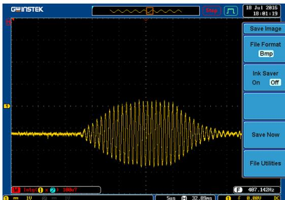
**Figure 21.** Received signal form PVC pipe
