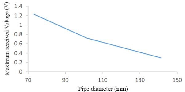
**Figure 11.** Effect of diameter on maximum received voltage
