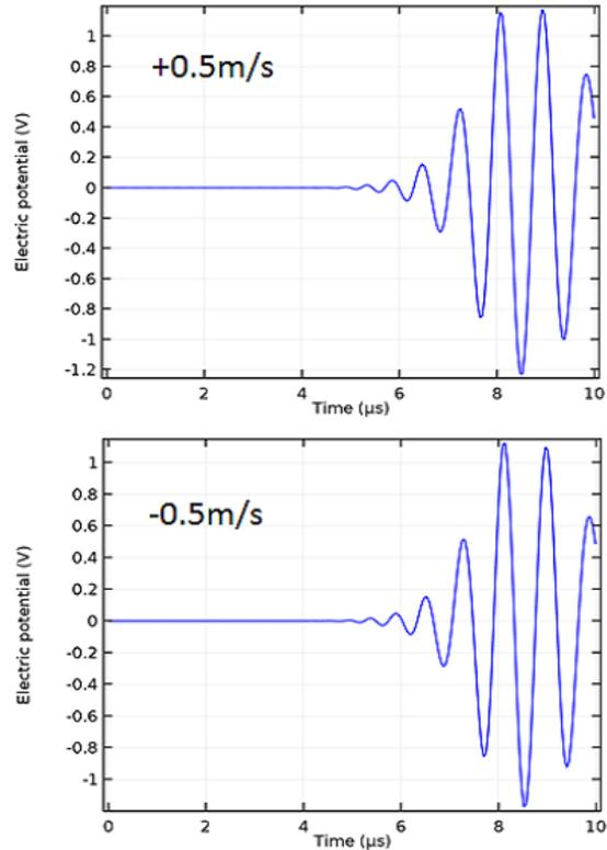
**Figure 10.** Received signal in dual opposite direction in DN65 pipe
