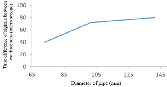
**Figure 12.** Effect of diameter on time difference between signals of opposite directions
