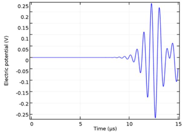
**Figure 4.** Received signal in sensor due to 12 Volt excitation signal
