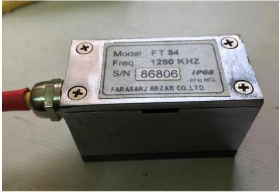
**Figure 17.** Sensor/transducer set for 1280 kHz frequency
