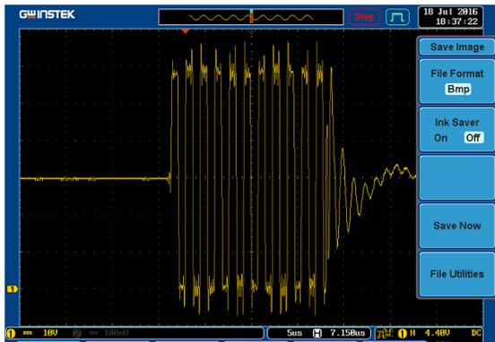
**Figure 18.** Excitation signal with 64 V amplitude
