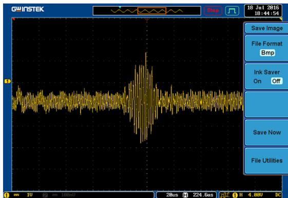
**Figure 20.** Received signal form asbestos-cement pipe
